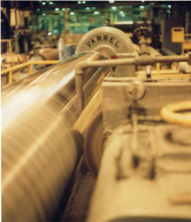
Pacer's special formula allows the wheel to act soft. The cork filler and rubber bond deadens any vibration because the abrasive grain is slightly cushioned. Grain is able to release more readily during light cuts. Pressure of the cork and rubber has a polishing action on the roll. Pacer cork wheels are heavy-duty and made to be run wet.
