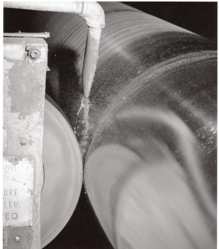
A dull wheel acts hard and can bounce on the roll. Machine vibration and wheel/roll harmonics also induce chatter. A spiral line around the roll is a product of a hard wheel face burnishing the roll. Abrasive grain pits are the depressions caused by loose grains (from wheel or coolant) crushed by wheel in to the surface. Variation of finish results from the changing condition of a glazed wheel face. Heat buildup is friction from flat grains rubbing on the hard roll.
